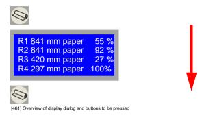
**Note:** The ROWE RS / RCS network printer can automatically detect the roll width. However, you will need to inform the device about the type of medium and remaining length nevertheless. You have to preselect the size of the inserted material if you do not have optional roll width detection since the device cannot identify this by itself. You do not however have to make any changes in the case that you are just changing an empty roll for a full roll of the same material.
