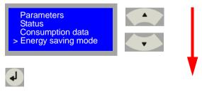
[438] Overview of the buttons to be pressed for setting the energy-saving mode.
