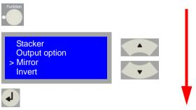
[153] Overview of the buttons to be pressed for enabling the 'Mirror' function.
