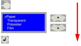
[68] Overview of the buttons to be pressed for selecting a printer medium
