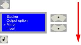
[88] Overview of the buttons to be pressed for enabling the Mirror function.
