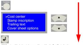
[98] Overview of the buttons to be pressed for enabling the Cost Center function.
