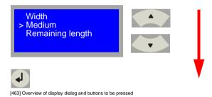
15. Using the arrow buttons 'Up/Down' [Fig. 464], select the desired medium and confirm your selection via the enter button. This will automatically save the medium selected and exits you from the menu.
