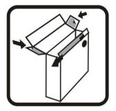
[489] Removing the protective films of the adhesive tapes
