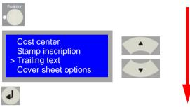
[96] Overview of the buttons to be pressed for enabling the Stamp / Trailing Text function.
