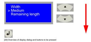
Using the arrow buttons 'Up/Down' [Fig. 21], select the desired medium and confirm your selection via the enter button. This will automatically save the medium selected and exits you from the menu.
