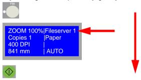
[138] Overview of the button to be pressed for scanning an original to file.
