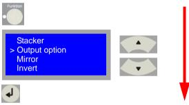
[100] Overview of the buttons to be pressed for setting the output option.
