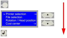
[65] Overview of the buttons to be pressed for selecting a printer
