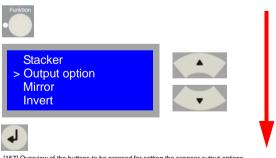
2. Using the arrow buttons 'Up/Down' [Fig. 158], select the desired state and confirm your selection via the enter button. The current selection will be stored and the menu automatically closed.
