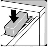
[480] Inserting the new toner cartridge
