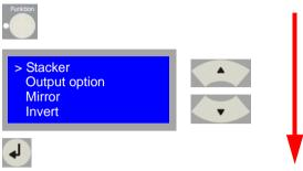
[80] Overview of the buttons to be pressed for setting the stacker.
