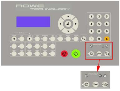
[119] Operator panel of network multifunction device ROWE RCS See chapter 2 from page 29 for the legend of the printer operation elements
