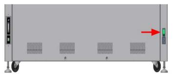
[2] On/Off switch on rear of printer
