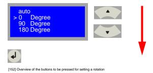
**Note:** When you select the menu option 'auto', the scanner will automatically rotate the file into the optimal space-saving position.
