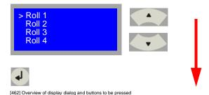
14. Using the arrow buttons 'Up/Down' [Fig. 463], select menu option "Medium" and confirm your selection via the enter button. This will get you automatically to the next menu level [Fig. 463]. You may abort the process and exit the menu by using the offline button.
