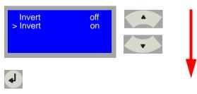
[156] Overview of the buttons to be pressed for enabling the 'Mirror' function.
