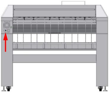
[40] On/Off switch on the rear of the ROWE RC network scanner
