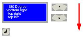
[79] Overview of the buttons to be pressed for setting the head position.
