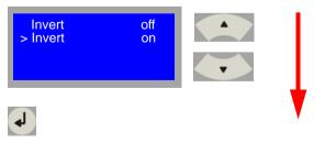
[91] Overview of the buttons to be pressed for enabling the Invert function.
