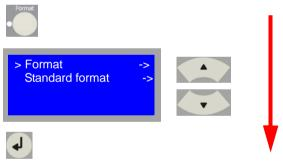
[71] Overview of the buttons to be pressed for selecting the input format
