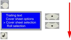
[92] Overview of the buttons to be pressed for enabling the Cover Sheet function.
