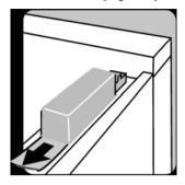
[481] Removing the sealing strip
