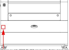
[12] Front view of the ROWE RS / RCS network printer. Position of mechanical counters
