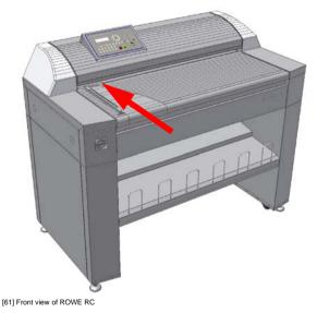
2. The scanner will run a 100 mm long prescan for width detection purposes provided the 'Automatic width detection' [p. 68] had been enabled. Then the original is returned to its start position. The scanner will now display the identified width [Fig. 62]
