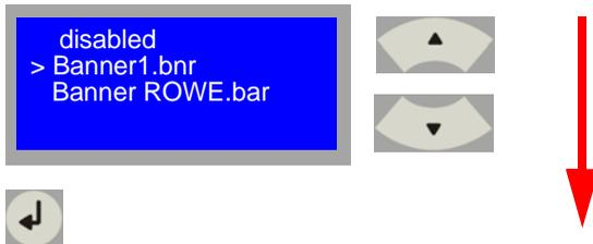
[93] Overview of the buttons to be pressed for enabling the Cover Sheet function.
