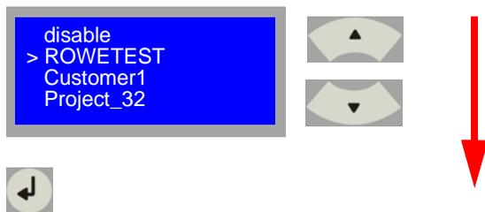
[99] Overview of the buttons to be pressed for enabling the Cost Center function.
